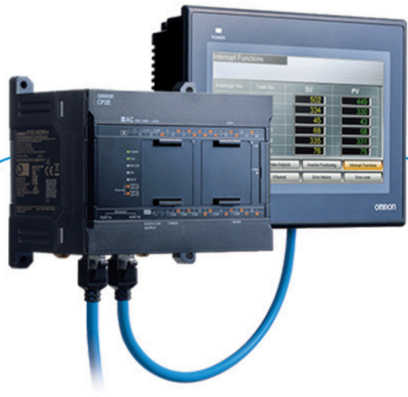
Programmable Logic Controller (PLC)
