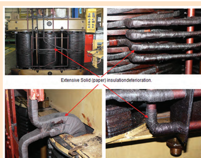
Figure 6: Deterioration of paper DP value <200 in the distribution transformer windings...
