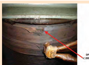
Figure 7: Showing effect of DP value<200 in a power transformer...
