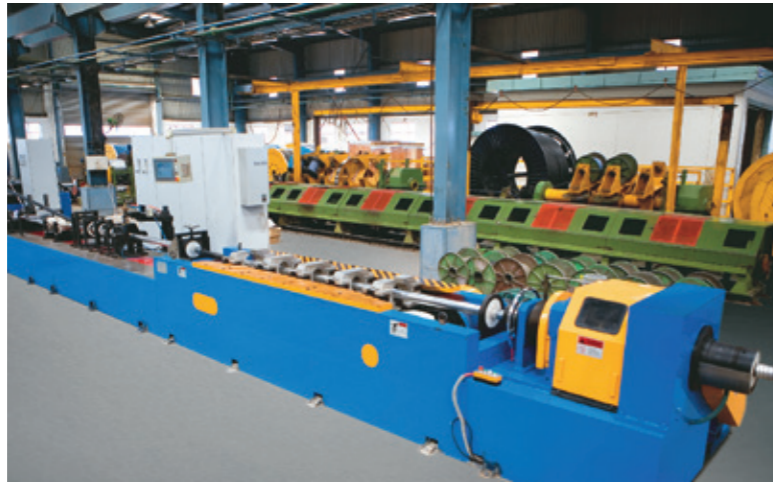
Aluminium Corrugation Sheathing Line
